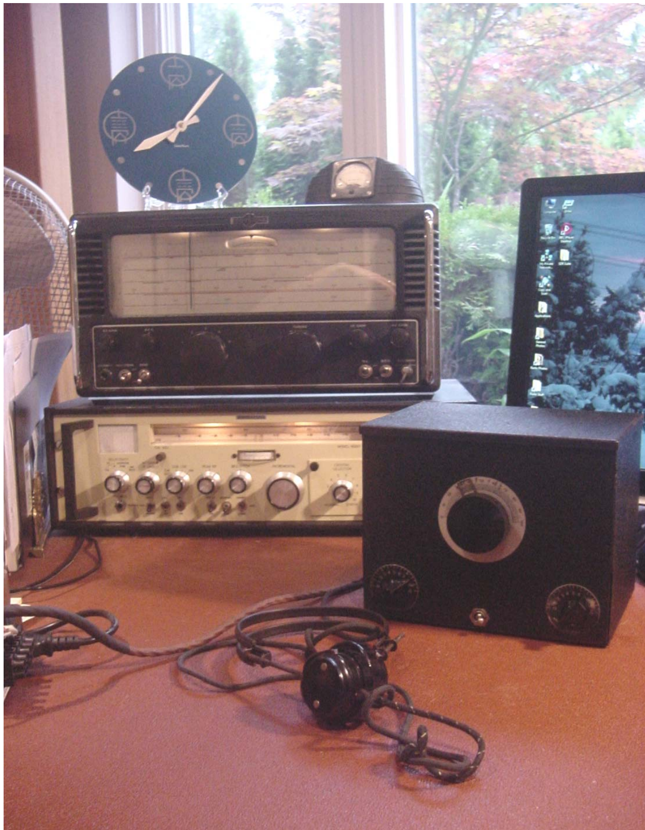
On-air comparison testing between the AW2 and my S.750 and Model 1830/1 receivers (borrowed high-impedance phones)
